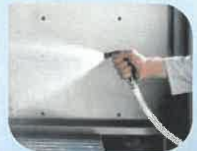
Hand-held coolant washdown gun for fast cleaning of workpiece
