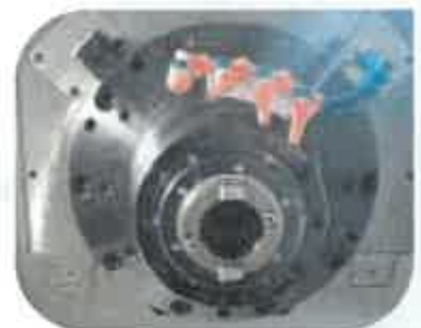
12,000 RPM spindle (ISO 40) with 4 adjustable coolant nozzles
