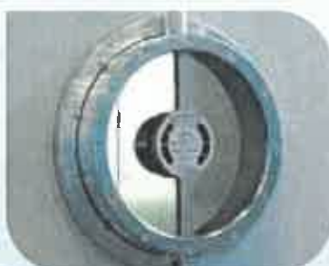
Rotating viewing window [VCP 600, VCP 800, UCP 600]
