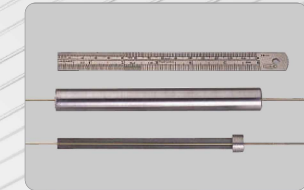
■ Deep hole drilling in ejector.
