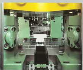
Tool loading area with view from the strip outlet side, with 2-part bolster plate and hydraulic tool clamping system (accessory).
