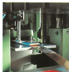
Strip guiding table with strip clamps for BRUDERER strip feed unit BBV 190/85 (view from tool loading area).
