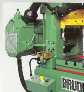
BRUDERER strip feed unit BBV 190/85, control panel for 2-hand operation (left side), and blow-out device (accessory).
