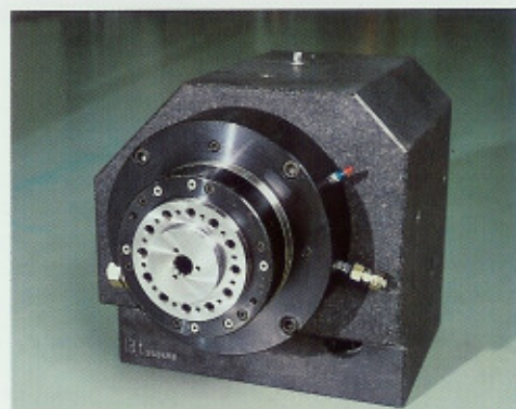
Hydrostatic main spindle, run-out \leq 0.1 \mu\text{m}
