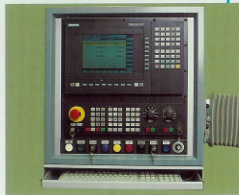
CNC-system, resolution 0.01 \mu\text{m}
